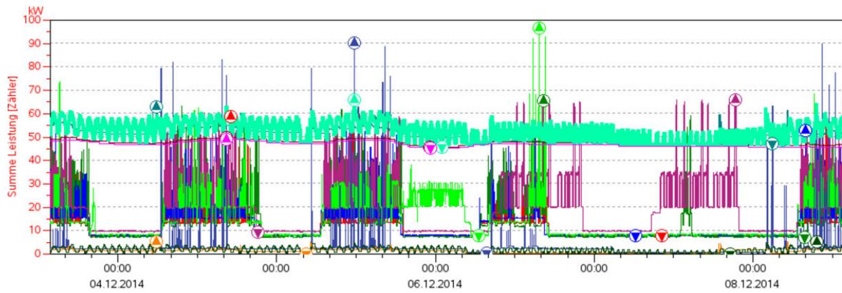
**Fig. 1:** Superimposed view of continuous energy consumption measurement of CT and MRI as well as climate control.
