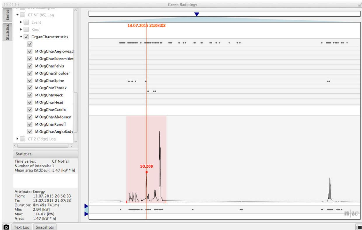
**Fig. 2:** Energy consumption of a patient scan. The different sized peaks represent scan events such as scout, pre-monitoring, spiral acquisition.
