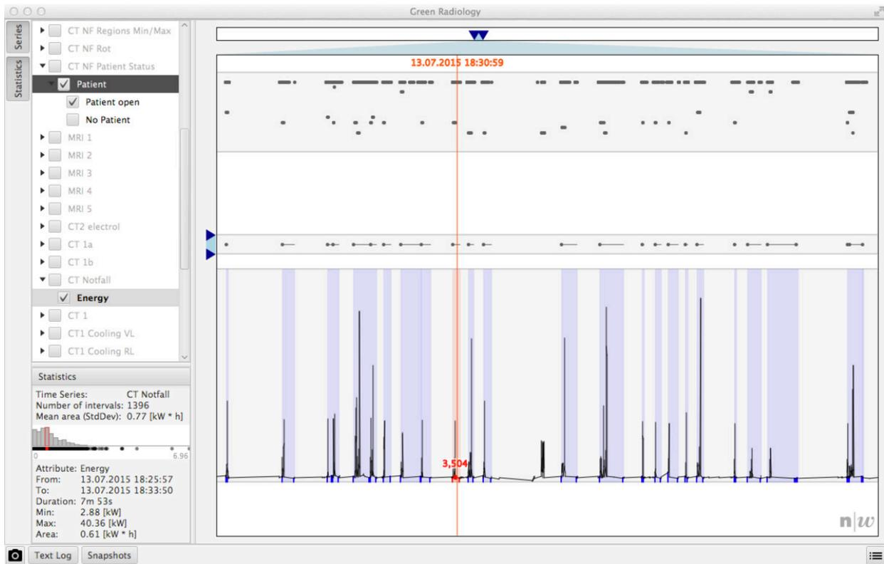
**Fig. 3:** Software allows for segmenting the continuous energy measurements into discrete events based on scanner log information and RIS events to calculate energy consumption e.g. patient room time.
